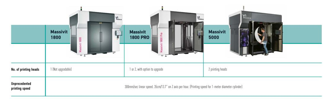
Experience unprecedented production speed for full-scale prototypes, molds, and parts. Massivit 3D printing systems comprise robust, large-volume hardware, easy, live monitoring via internal cameras and computer vision, user-friendly software, advanced slicing algorithms, and a range of photo polymer materials.
